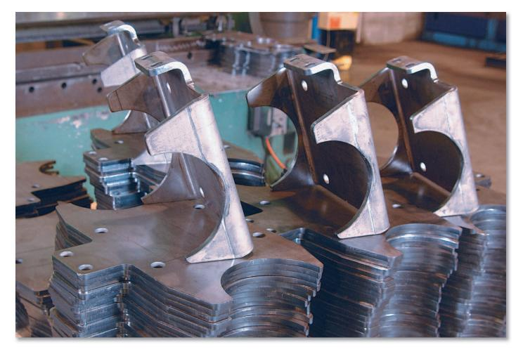
On the Whitney 3400 XP, the production cycle is automatic and complete. Raw steel is loaded and positioned by the PartHANDLER-II automation system. Parts are punched and plasma cut by the 3400 XP. Small finished parts are removed automatically using a drop door; larger parts are offloaded by the PartHANDLER-II using programmable magnets. A large drop table removes the completed skeletons while production continues, uninterrupted, on the next plate.
